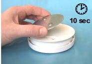
Take the magnetic base element, pull the protective foil off and ad-here it to the assembly plate of the smoke alarm. Press down firmly and hold it for at least 10 seconds.
